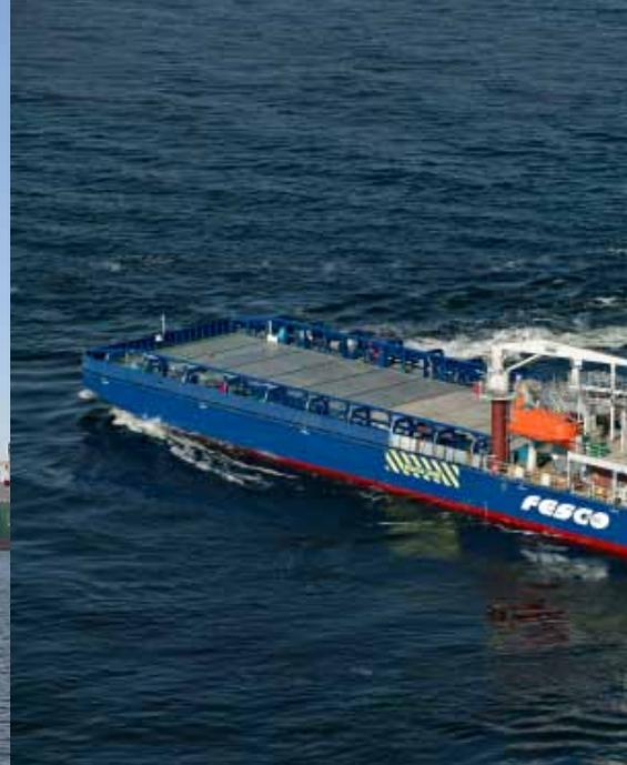
The FESCO Sakhalin Ice-breaking Supply and Standby Vessel is equipped with three Wärtsilä 8L38 engines
