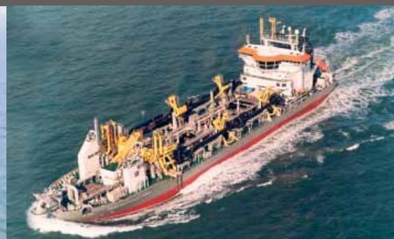
The trailing suction hopper dredger Prins der Nederlanden of Westminster Dredging Co. Ltd, a 100% subsidiary of Royal Boskalis Westminster nv, is equipped with two Wärtsilä 12V38 engines and one Wärtsilä 9L20 engine.
